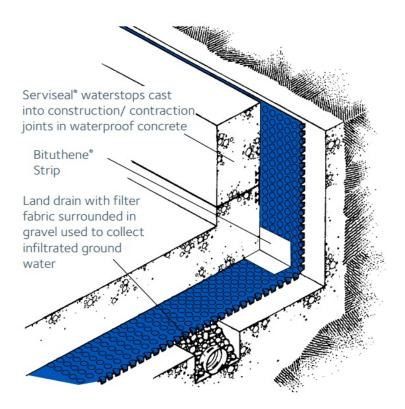
Typical section through underground structure with Hydroduct CF20 Cavity Former used to line excavation and collect infiltrated water
