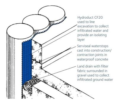
Typical section through structure with piled wall
