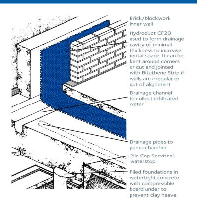
Hydroduct CF20 used within sandwich construction to form a drainage cavity and collection layer which maximises rental space
