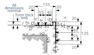
Serviseal Pilecap can be used around pilecaps or column bases or in joints at internal angles of retaining walls and linked with other Serviseal waterstops.
